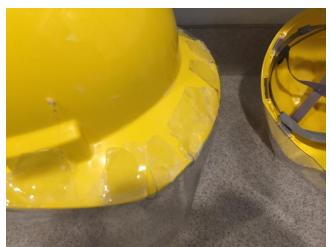
In the first prototype that I made, I crenelated the top of the plastic so that it would glue easily on to the rim of the hard hat. But this made the plastic sheeting to come too close to the face. It was hot and fogged up too easily. In the second prototype, I glued the sheeting as shown. It doesn't look as 'nice' but it made the face shield be further away from my face. It was more comfortable to wear.
