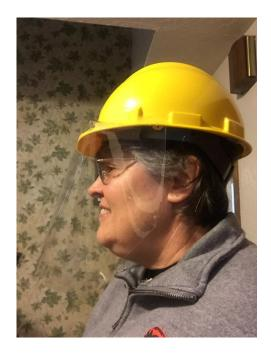
I cut the plastic to about  $16 \times 10$  inches and beveled the sides. Otherwise they bump the shoulders and displace the hard hat.
